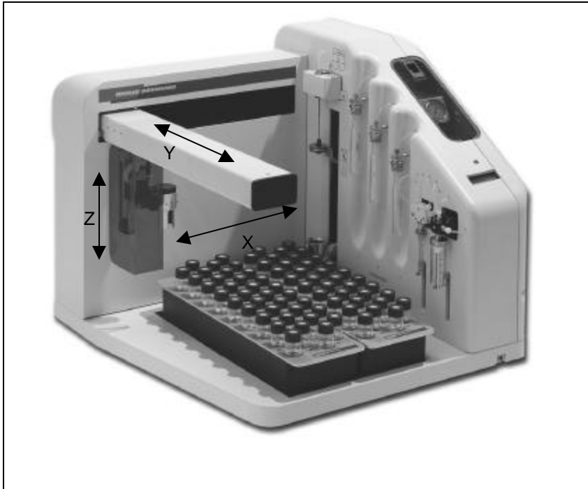
Figure 1-7: Robotic Arm Movement (X, Y, and Z)
